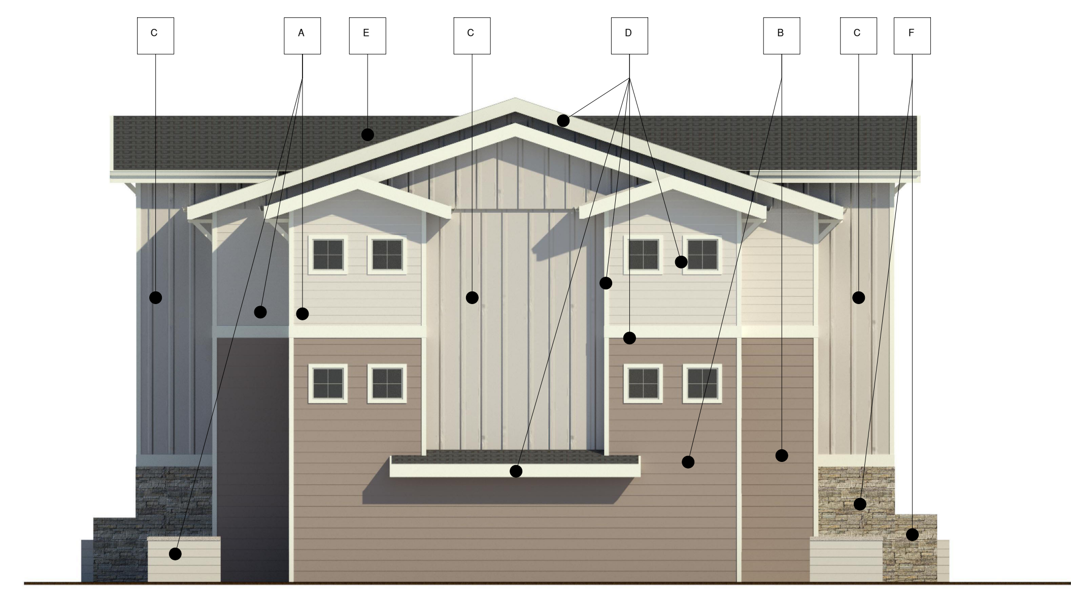
2 BLDG. TYPE A - LEFT ELEVATION 3" = 1'-0"
